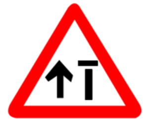
LANE CLOSED (ON A TWO LANE ROAD)
