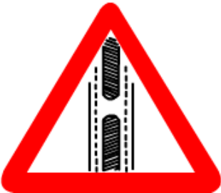
GAP IN MEDIAN
